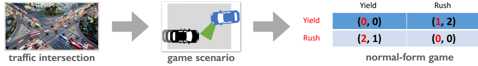
Figure 19.3.1 A snapshot of stochastic time in the intersection example. The scenario is abstracted such that there are two cars, with each car taking one of two possible actions: to yield or to rush. The outcome of each joint action pair is represented by a normal-form game, with the reward value for the row player denoted in red, and column player denoted in black. The Nash equilibria (NE) of this game are (rush, yield) and (yield, rush). If both cars maximize their own reward selfishly without considering the others, then they will end up with an accident
